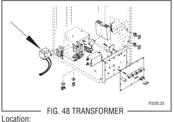
The transformer is mounted on the side of the tank mounting bracket for models 3.4 & 5. The transformer is located behind the lower front access cover, mounted on the rear side of the component bracket for models 3S.3S+.5S & 5S+.
