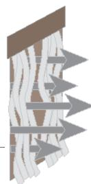
Plastic Strips Allow air, smells, contaminants, climates and bugs to pass through easily, while hindering employee movement.
