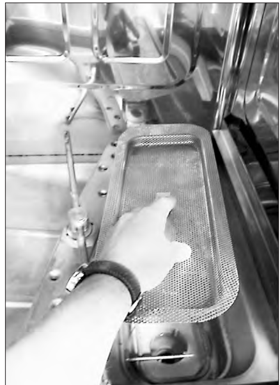
Make sure the scrap screen is in place.
