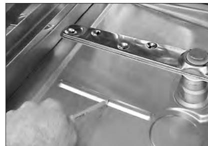
Proper Water Level in the Wash Tank.
