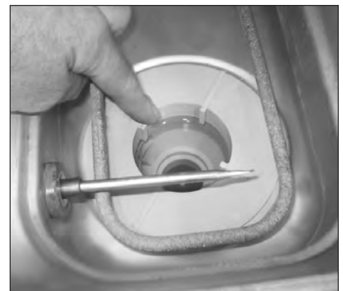
Clean the pump intake screen
